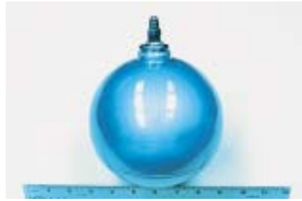
Spherical pressure container with PhotoStress coating applied to entire surface area.
