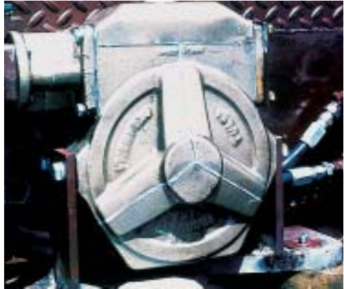
PhotoStress coating applied to the cast housing of a hydraulic drive system of a fire engine.
