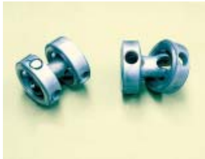
Newly designed universal joint coupling coated and ready for PhotoStress testing.
