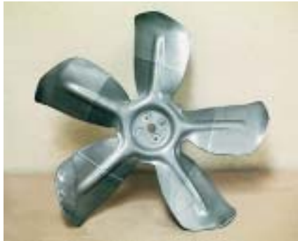
PhotoStress coating applied over the entire surface of a fan which was dynamically tested.
