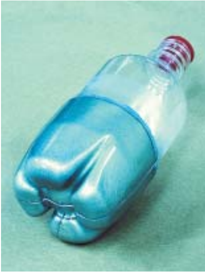
A plastic beverage bottle coated for comparison of PhotoStress and finite-element analysis.
