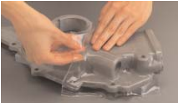
PhotoStress coating being contoured to the surface of a vehicle water pump casting.
