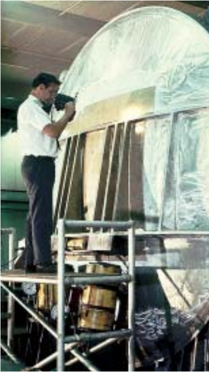
A large pressure container with PhotoStress coating applied to a “ribbed” reinforced area.
