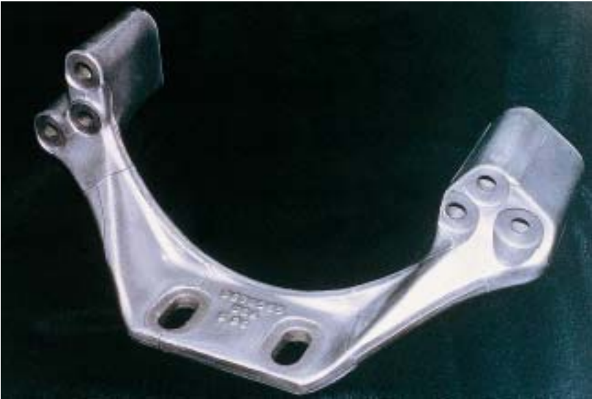
Engine mount bracket with PhotoStress coating bonded in place. Coating covers entire surface except in the immediate area of the bolt holes, and other areas where fasteners and completion hardware would physically come in contact with the coating.
