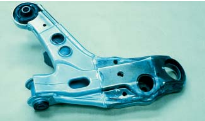
An automotive control arm bracket partially coated for PhotoStress analysis.
