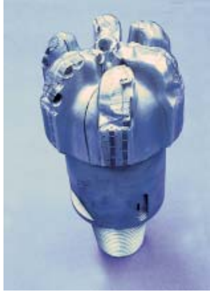
PhotoStress coating applied to an exploratory oil field drill head.
