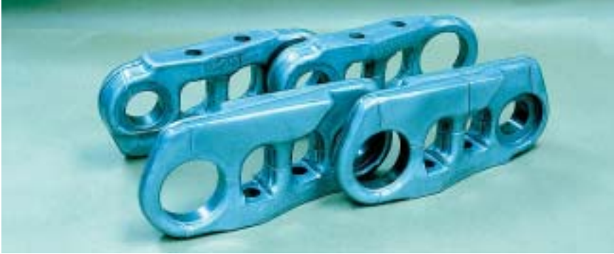
PhotoStress coating applied to track links from an earth-moving vehicle.
