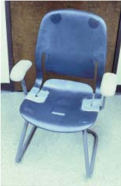
Chair showing coating applied to areas of seat which was designed for greater flexibility.
