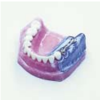
PhotoStress coating applied to a dental model used for design of bridge components.
