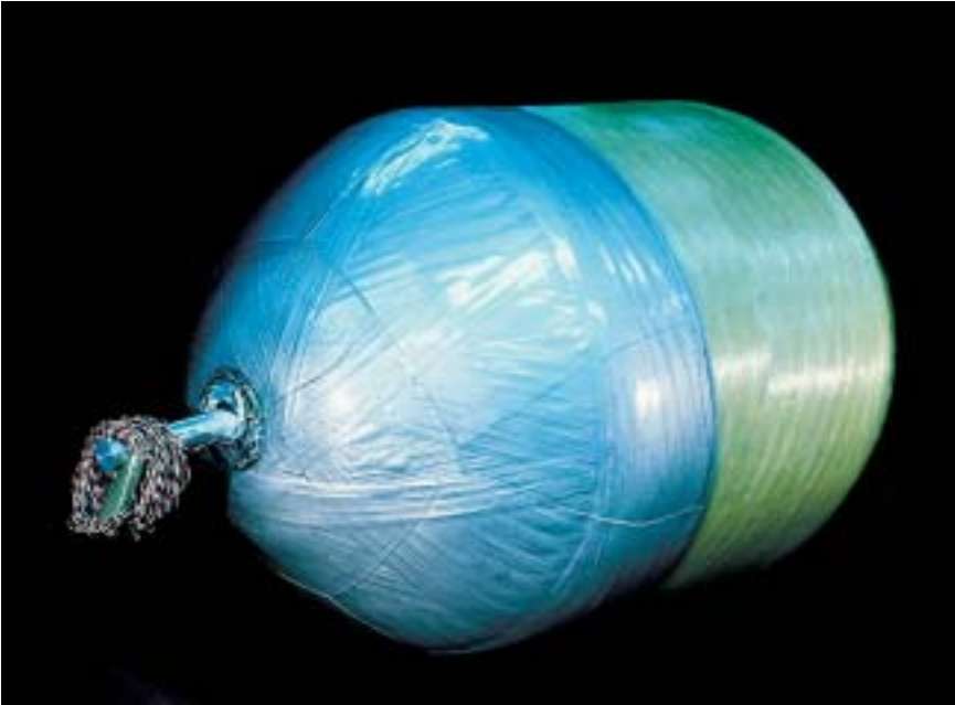
Filament-wound pressure vessel partially coated for testing. PhotoStress coating can be applied to any material regardless of its homogeneity.
