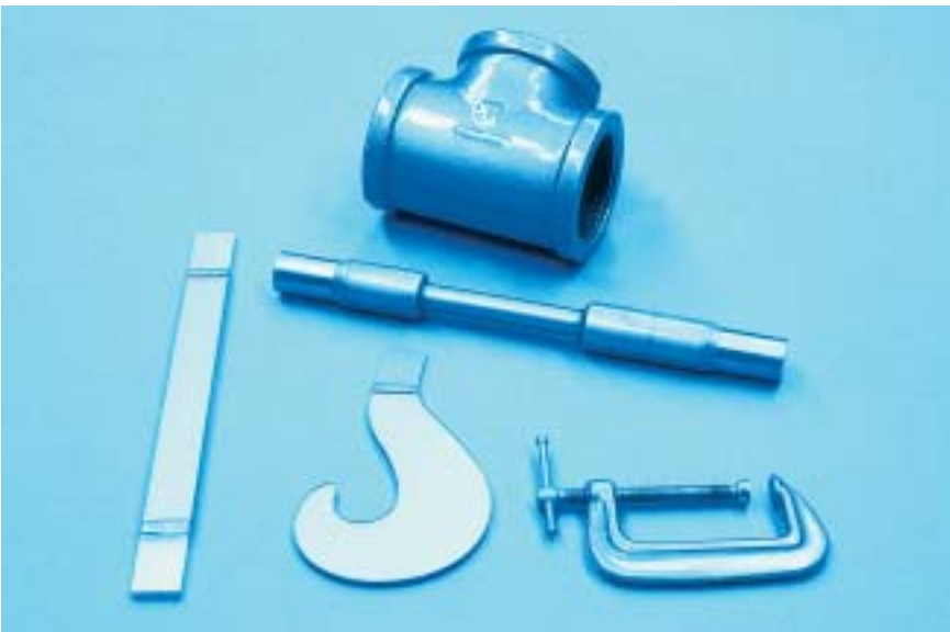
Typical samples that have been coated for conducting student experiments in PhotoStress testing at colleges and universities.
