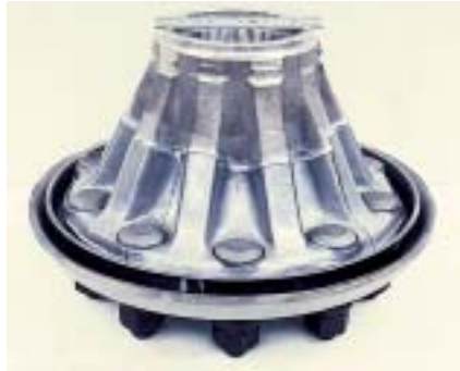
PhotoStress coating applied to rapid transit vehicle wheel hub.
