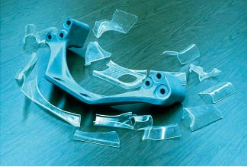
PhotoStress contoured shells ready for bonding to engine mount bracket casting.
