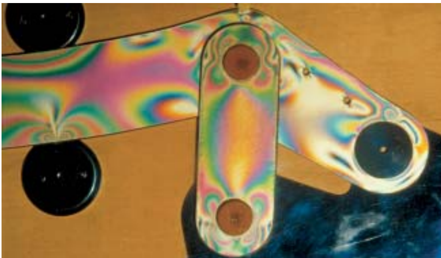
Fig. 1—PhotoStress pattern revealed on a mechanical controlled linkage system in a passenger jet aircraft.
