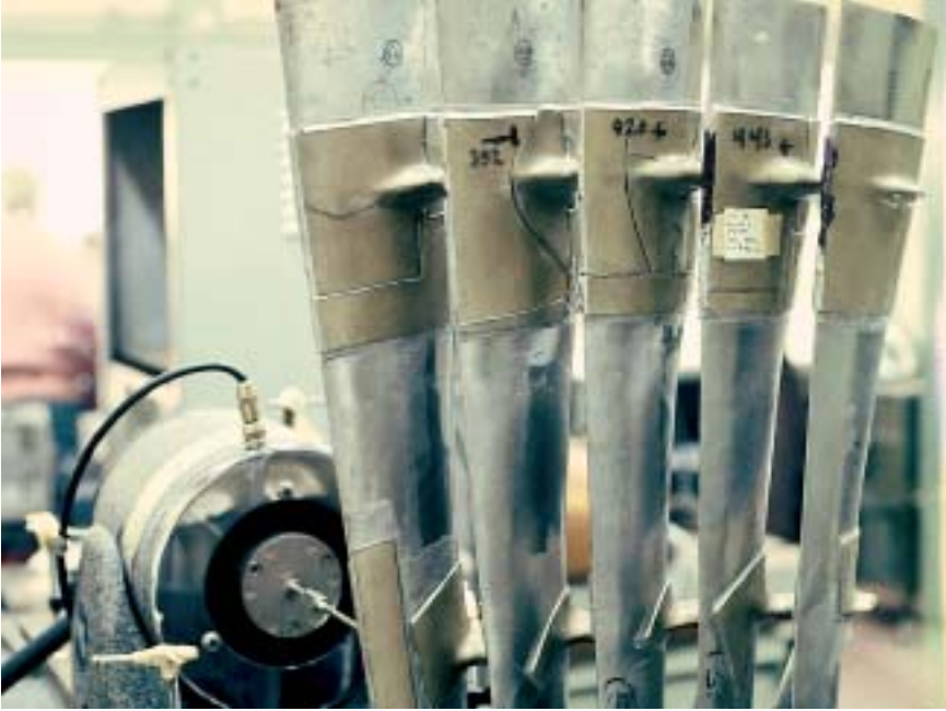
A section of steam turbine blades coated for PhotoStress analysis under dynamic test conditions.
