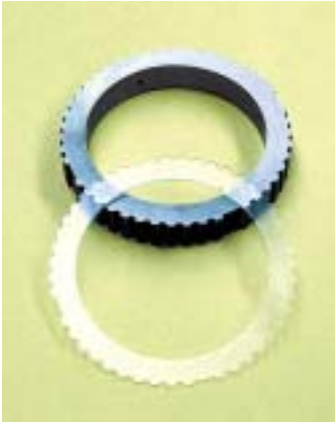
Coating ready for bonding to geared ring.
