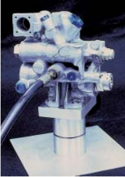
PhotoStress coating applied to a complex shaped augmentor fuel casting from a jet engine.
